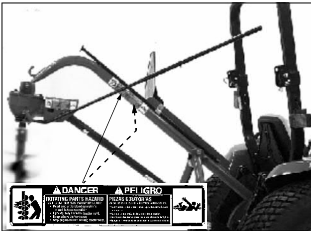
Picture Note: The safety label is on both sides of the boom.
