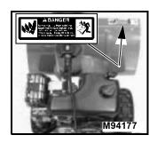
**DANGER** - ROTATING BLOWER. Shut off engine before unclogging discharge chute.
