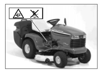
DO NOT drive where tractor could slip or tip. DO NOT drive on a slope with more than a  $11^{\circ}$  (19%) incline.
