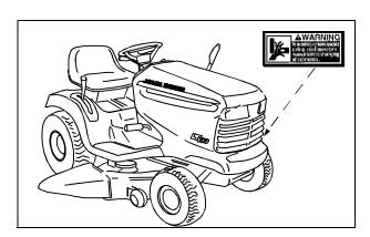
Picture Note: Label is located on Left-Hand Side of Tractor Frame with 48C Deck and when Optional Lift Assist Kit is installed on 38-Inch or Freedom42 Deck
