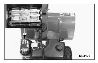
The word HOT is embossed in the muffler shield.
