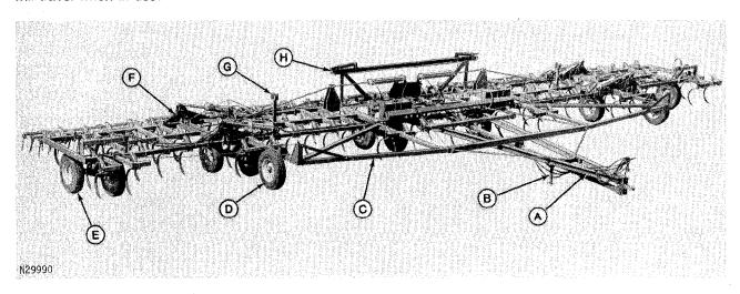
A-Hitch B-Jack C—"A" Frame D-Stabilizer Wheel -Tandem Wheels
