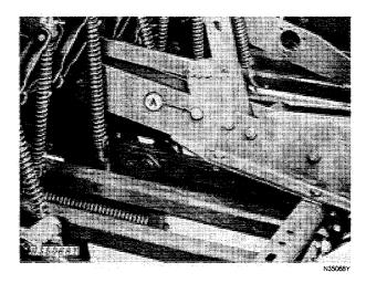
Always raise the openers and install locking pin in transport position (A).
