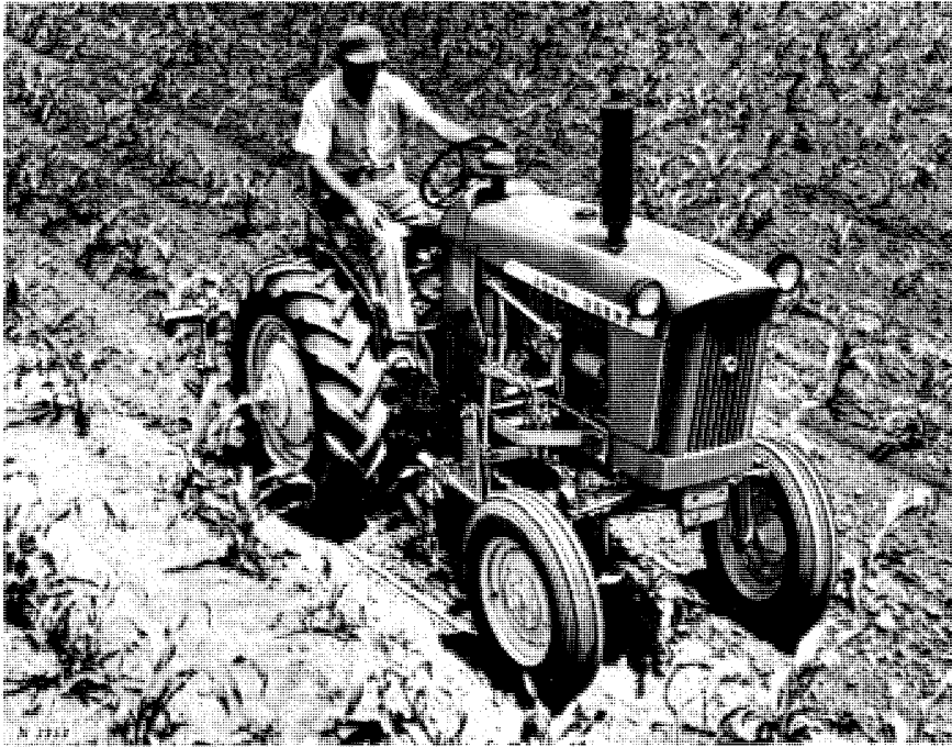
Right-Hand View of John Deere S1 One-Row Row-Crop Cultivator
