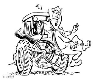
PTO master shield should be in place at all times except when connecting a PTO drive line or for special applications as directed in the operator's manual.
