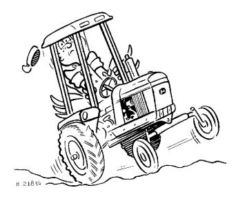
Slow down for hillsides, rough ground, and sharp turns. Couple the brake pedals together before driving at transport speeds.
