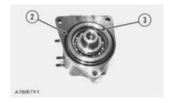
2. Remove O-ring seal (2). Remove snap ring (3) with tool (A).
