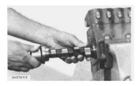
**3.** Install the rack bearing in the accessory drive end of the housing with tooling (D).
