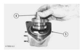
**3.** Put shaft assembly (4) in position in housing (5).
