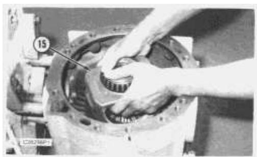
**18.** Put center housing (23) in an appropriate support fixture with the open side facing upward. Lower differential group (15) and bevel gear into position in the center housing.
