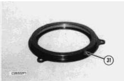
**26.** Remove O-ring seal (31) from the piston.
