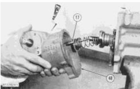
16. Put the gasket and governor housing (48) in position on the fuel injection pump housing with bolt (17) and the spring seat in alignment with the spring guide in the governor housing. Install the bolts that hold the governor housing to the fuel injection pump housing.
