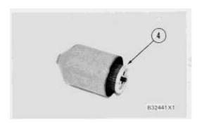
**3.** Remove element assembly (4) from the case.
