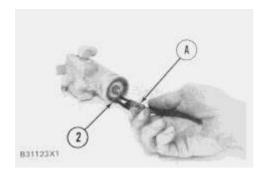
2. Remove snap ring (2) with tooling (A).
