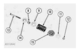
**4.** Install retainer (14), spacer (8), retainer (9), spring (11), nut (15), washer (11) and jam nut (12) on bolt (13).
