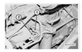
1. Remove two tube assemblies (1) and (2) from the air compressor governor.
