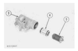
**3.** Remove spring assembly (5) and piston assembly (4) from the governor housing (3).
