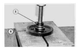
**5.** Install the bearing in idler gear (4) with tool group (A) and a press. The end of the bearing must be 1.52 mm (.060 in. below the face of the gear hub.
