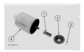
1. Put spring (1) and retainer (2) in place in case (4).
