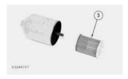
**3.** Put element assembly (5) in position in the case.
