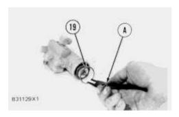
**6.** Use tooling (A) to install snap ring (19).
