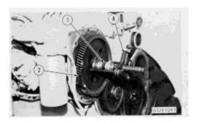
2. Remove bolt (1) and the washer that holds gear (2) in place.
