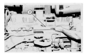
**3.** Install the spacers and heat shield (2).
