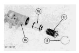
**5.** Put piston assembly (16) and spring assembly (17) in position in housing (18).
