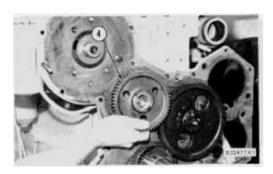
**6.** Put idler gear (4) in position. Install the plate and bolts.
