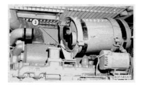
**4.** Install bracket (3) and the bolts that hold it in place. end by:
