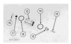
6. Remove pin (15), spring (19), retainer (17) and spring (16) from the piston.
