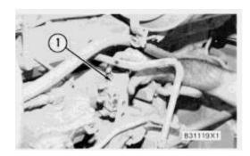
1. Put governor (1) in position and install the two bolts that hold it to the bracket.
