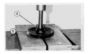
7. Inspect the bearing in idler gear (5) for wear or damage. If a replacement of the bearing is needed, use tool group (B) and a press to remove it from the gear as shown.
