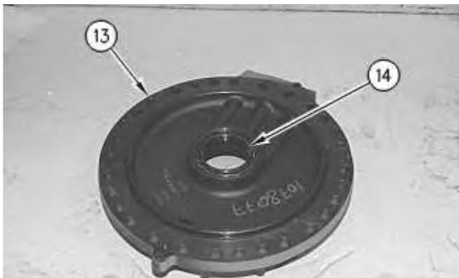
9. Install bearing (14) into housing (13) .
