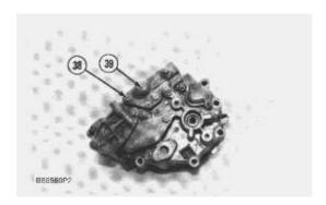
13. Remove two bolts (38), cover (39) and the gasket from the housing.
