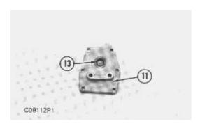
**6.** Remove seal (13) from cover (11) with tooling (B).
