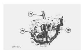
10. On earlier engines, remove shaft assembly (28), lever (29) and lever (30) from the housing.
