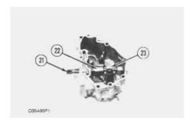
c. Remove shaft assembly (21), lever (22) and lever (23) from the housing.
