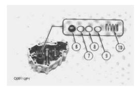
**4.** Remove governor spring (10), two wave washers (7) and (9), one flatwasher (8) and seat (6) from the guide.
