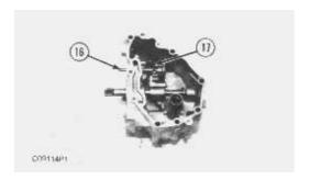
**8.** Remove shaft (16) and lever (17) from the housing. Remove the ring from the shaft if necessary.
