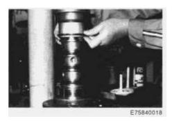
**3.** Install O-rings (10) into the O-ring grooves on inside body (11) while moving inserter B from the low position upward.
