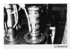
6. Apply grease onto O-ring (10) and backup ring (9) with brush.
