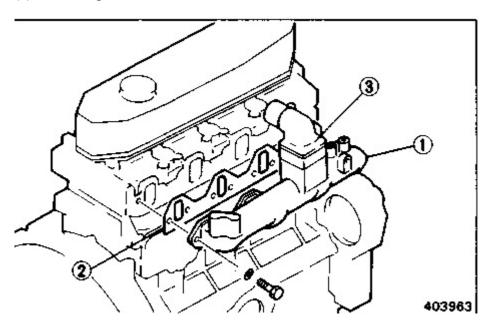
Unscrew the bolts securing inlet manifold (1), and remove the manifold and gasket (2) complete with air heater (3).
