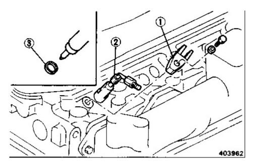
Take off nozzle gland (1), and remove injection nozzle (2) and gasket (3).
