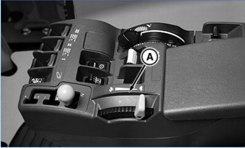
RXA0070892-UN: Current Version Armrest with Raised Throttle Guard
