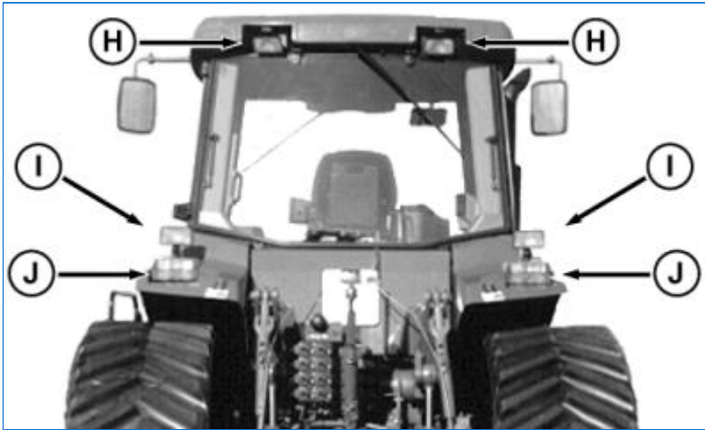
RW56482A-UN: Rear Roof and Fender Flood, Tail Lights
